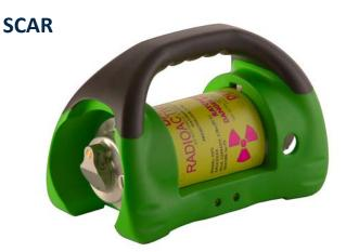
AMSYCO owns and operates the latest SCAR equipment which is ideal for shutdowns and for carrying out radiographic work in heavily congested work areas. The SCAR system permits the performance of radiography within a confined controlled area without disruption to normal operations. We are licensed to import and operate Selenium 75 sources.
